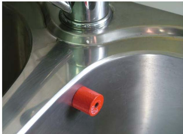
The strength of the magnetism depends on how much the metal has been deformed. Even when these grades are cut (cold, by shearing) the deformation in the edge of the metal causes magnetism.
