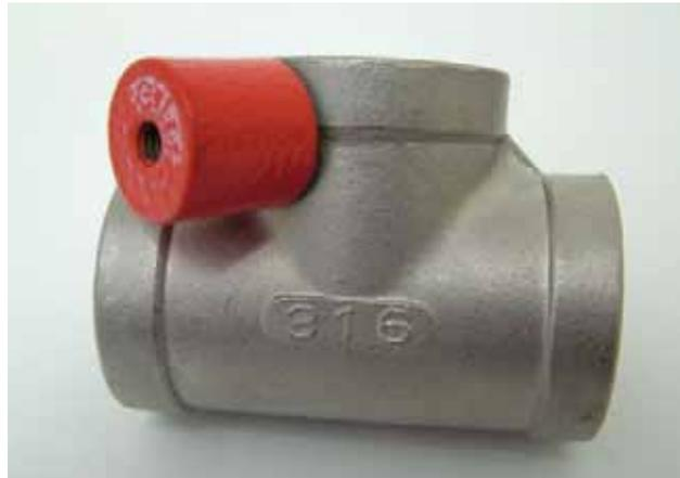
Cast austenitic grades are likely to crack in the casting process if they aren't formulated to be somewhat magnetic – the same applies to welds. So castings are usually magnetic, unless they have been heat treated.
