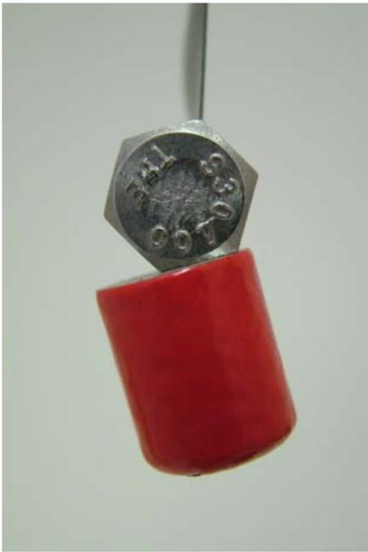
Stainless steel bolts are made by cold forging the head, and cold rolling or machining the thread. They are often quite strongly magnetic.
